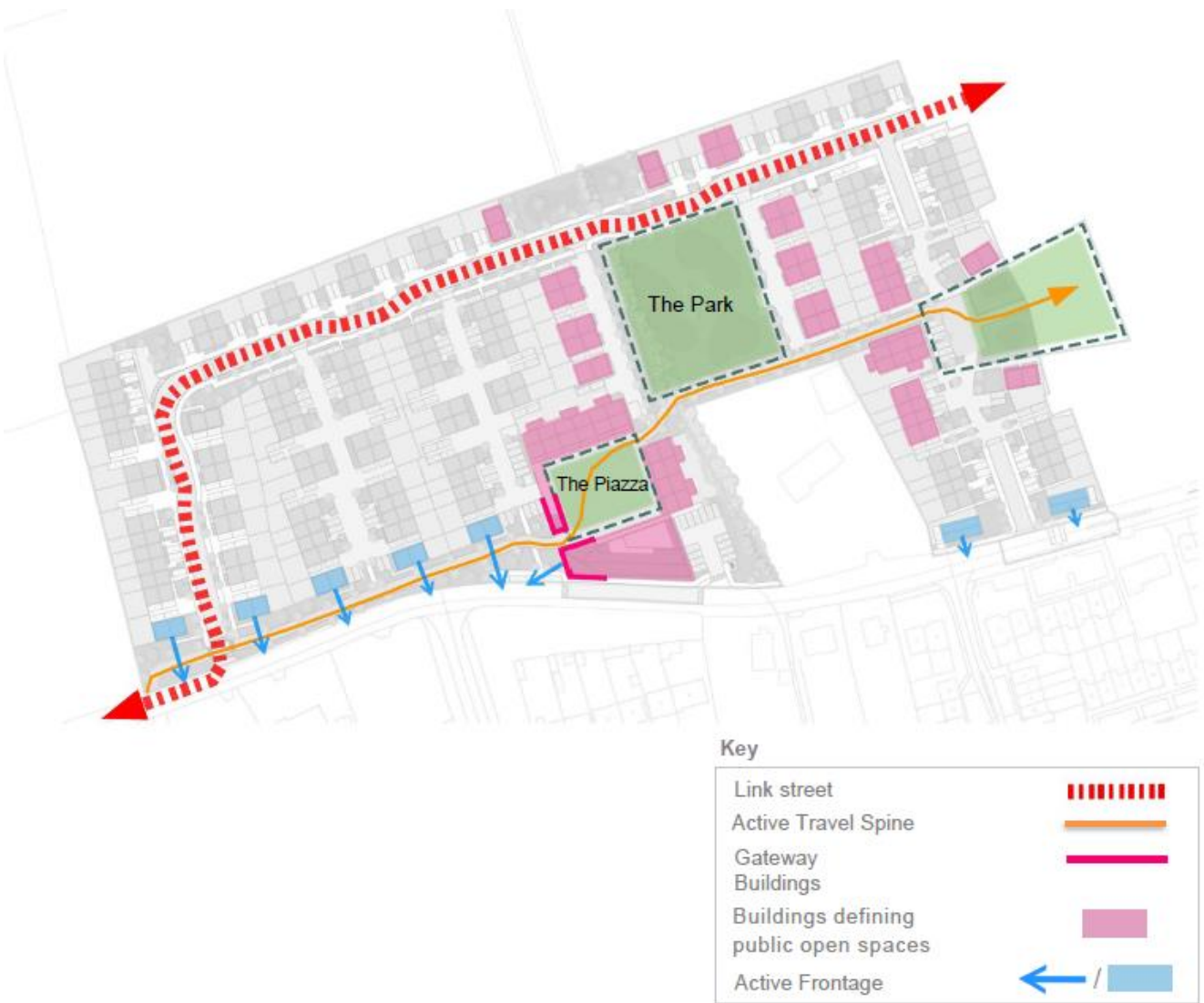
Figure 5.2: Diagram illustrating the principal layout elements of the Proposed Development. Source: JFOC Architects.
